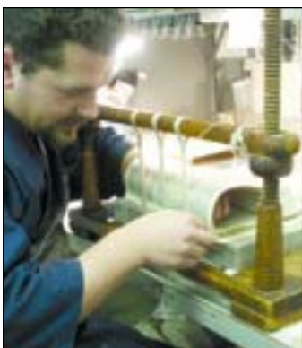
Conservator sewing new binding.
